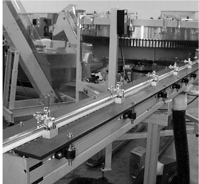
Several Model 201-U clamps, with hex-head spindles, are used to secure a guide in a bottle capping application.
