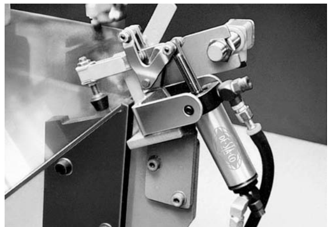
Model 817-U on a pneumatic clamping fixture
